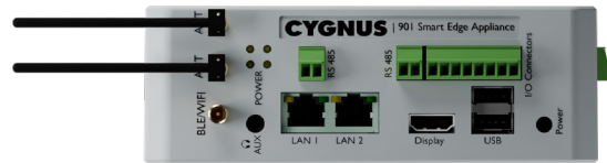
Versatile connectivity USB 2.0, Ethernet (RJ45), RS485 & HDMI
